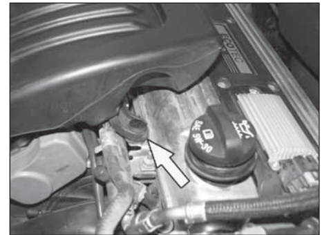
8. Unclip air box mounting clip.
