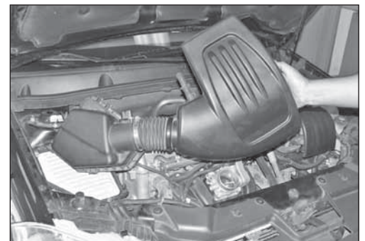
9. Lift firmly upwards and remove air box from vehicle.
